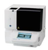
i-densy provides easy SNPs analysis of your choice. Fully integrated automatic system from Pretreatment, amplification, to detection.
