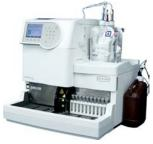
HA-8180T incorporates unique HPLC column technology to make it the fastest analyzer of HbA2 in the world. This model is highly effective for  $\beta$ -thalassemia testing.
