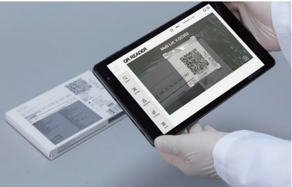
By reading reagent information with a mobile device, calibration can be performed.
